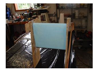
After cutting off 1" from each of the saddles (length) Use 5 minute epoxy to glue them to some plywood. Add a ½" wide wood strip to the trailing edge of each of the saddles flush with the foam surface. This will extend the saddle to cover the tubing and layup thickness that you've added to the foam blank.
