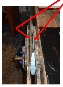
Using the stands used for making your rudder and centerboard, bond the blank (leading edge facing up) to the stands. Use 5 minute epoxy and some long wood screws to hole the foam in place
