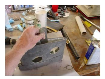
Now is a great time to bore the pintle hole out to the correct size (5/16"). You'll need a 12" long bit for your drill press. The hollow carbon batten that you used provides the perfect pilot hole and will keep the bit centered. Use a plane blade or knife (and a lot of cussing) to peel the cloth and peel ply from inside the body. You should never sand this inside surface because the peel ply leaves a good bonding surface for the Spartite fill that you'll use to make the rudder gasket.
