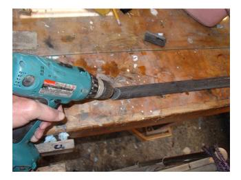
Drill a 5/16" hole on a 45 degree angle starting near the top of the filler. Be sure to have the tiller setting on wood backing to avoid fracturing the carbon fibers around the exit hole in the bottom of the tiller.
