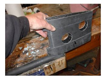
Begin by setting the body on the tiller and scribing the inside of the body onto the tiller. Cut to these inside lines. Use a sanding cylinder to begin the trial and error fitting process—constantly sanding and sliding the tiller further onto the body
