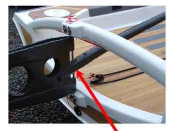
To get it right there are a few constants that you need to know. First, the transom bottom gudgeon block is 3/8" below the deck top at the transom. Second, the transom bar was made following the instructions in the manual and is flush with the transom (72" radius). Third, The toe rails are standard height. Use this gudgeon-less system as it has been tested and proven over nearly three seasons of hard sailing
