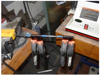
Clean up your plywood stands and glue the cassette back on to the stands. Put masking tape on the cassette body so that the outer edges are 4" apart (leave 2  $\frac{1}{2}$ " on each end). Glue a  $\frac{1}{4}$ " x  $\frac{1}{4}$ " rib on the centerline of the leading edge. I have some s-glass and hybrid stock made up that is  $\frac{1}{4}$  inch thick that I use for this kind of application. Do not adhere the rib between the tapes
