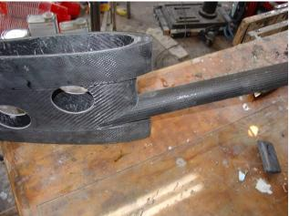
During this process you can guess the approximate amount of tiller angle. After fitting the tiller, dig the foam out of the tiller about 1 ½" past the nose of the cassette body. You will fill this cavity with filler later
