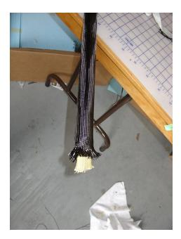
Cut one full length piece plus 3" of both carbon and Kevlar. In addition, cut an 9" and a 12" piece for the ends. Use the 12" piece on the small end since you'll be bolting the extensions in this area
