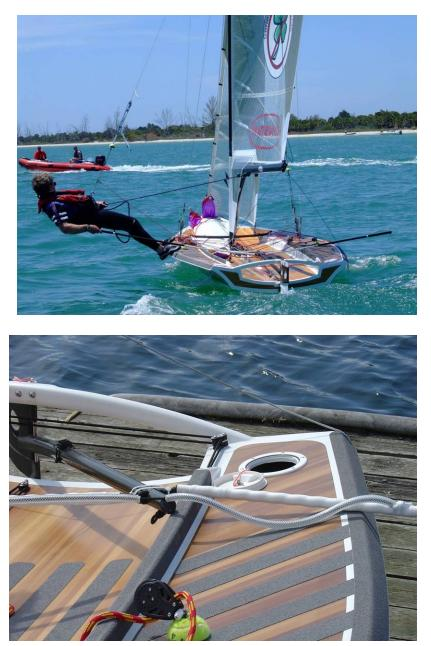
The tiller angle is pretty important. If the tiller extension attachment point is too low, it will cause the extensions to cause issues with the toe rails when tacking. If it is too high, the outer end of the extensions will be more likely to drag in the water—especially during tacks and gybes.
