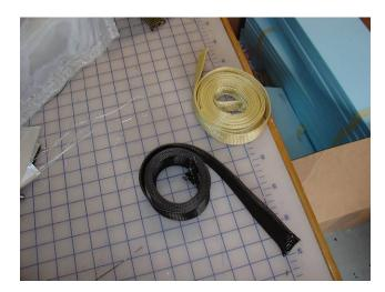
Above you see both Kevlar and carbon sleeve. Above left is the foam core for the tiller. Slide the sleeve over the foam core to measure the amount of each needed.
