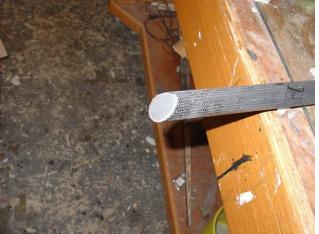
Use a screwdriver or drill bit to clean out about 2" of foam from the end of the tiller. Sand the inside a bit and clean with a paper towel and some acetone. Fill this space with a mixture of epoxy, silica, and a bit of carbon powder (heavy cream consistency).
