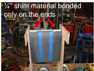
Fillet and fair the carbon wrapped batten on both ends. This may take a couple of applications since you'll want to be sure the batten is centered and true with the cassette so your rudder will be vertical.
