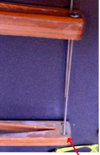
The angle of these inserts is critical to allow the rod to hook up with the threads in the lower cassette
