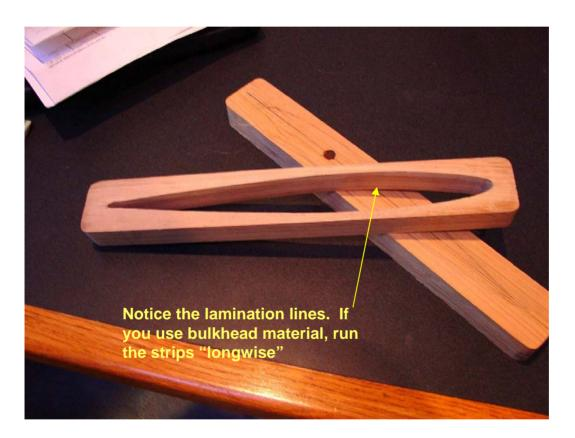
Cut the cassettes slightly oversized and bevel the edges with your disc sander by setting the table at 4 degrees. This will make a wedge shape that will make the insert tighter as it is inserted further. Leave a little space since you'll want to wrap the edges with 1" glass tape and epoxy. Use a little silica when you coat the glass cloth so you can re-sand it to make the block fit tight.
