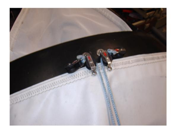
4. After locating the jib block attachment holes, install the velcro strip in a straight line from one edge of the throat to the other.
