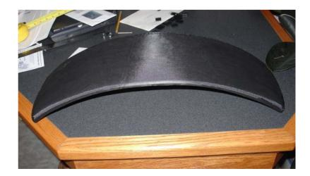
The finished launcher throat weighs 1 lb.
