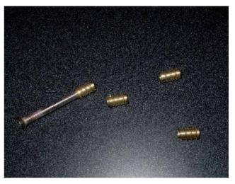
After the launcher is installed on the boat, you will install these brass inserts for the jib blocks. The holes should be drilled oversize (3/8" for 1/4" OD inserts) and the inserts bedded completely in epoxy. Drill the depth until you feel your bit hit the bottom skin of the launcher. Do not install these block until you have the spinnaker sock ready to install.
