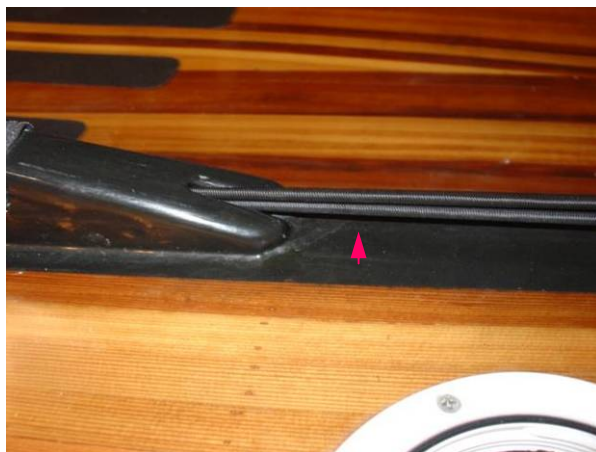
The bottom shock cord is the trapeze cord from this side and the top one is from the other side (it will go forward to the righting cord)
