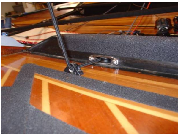
Shock cord enters sheave and toe rail tunnel where it turns aft
