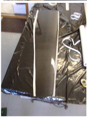
Normally, I use fairing filler/silica/graphite powder on centerboards to finish them up. You'll want your rudder to be white (two part linear polyurethane) so you can see weeds on it (you can't see you CB so it doesn't matter that it is black)
