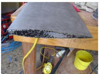
Left you see the top filled. It is then sanded flat and a piece of flats stock can be put on top for cosmetics. Below the flat stock was about 1/8" and beveled at the top to get rid of the sharp corner.
