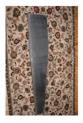
After you trim the trailing edge, cut the tip off square and the head at the angle of your deck (slide it in your trunk and mark it). Keep the blade as long as possible unless you are quite light or normally sail in heavy air. Even then, never cut it down more than 5 inches from the original blank length because you can raise it about 8 inches before it interferes with your vang and sail cheeks.
