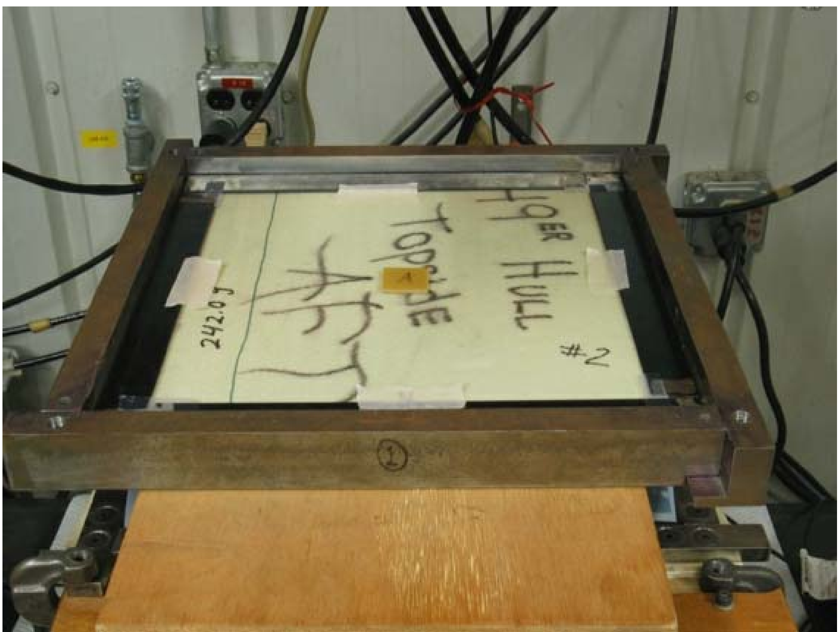
Panel #2 (49er) installed in the lower panel edge-support frame.
