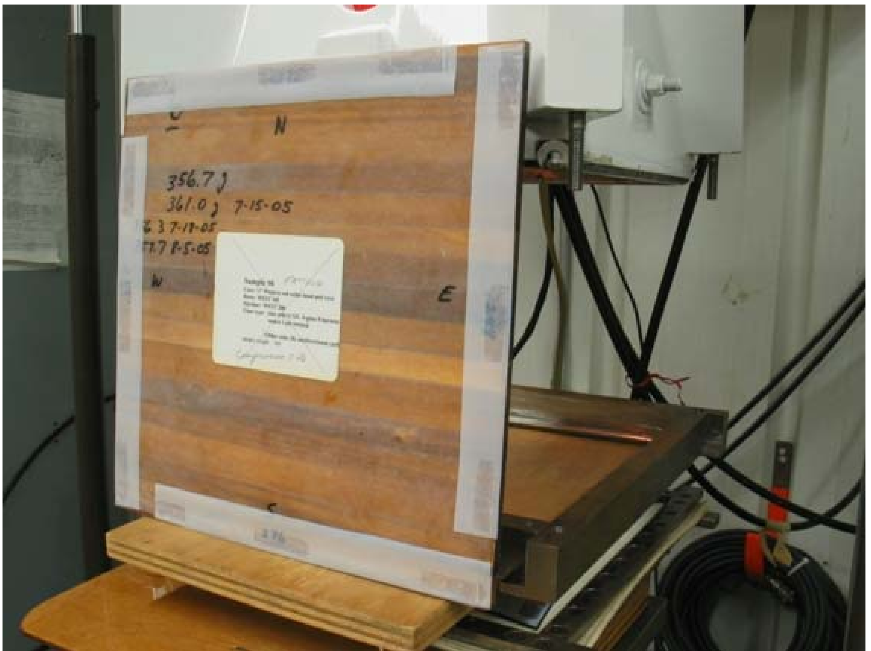
0.005-inch-thick Teflon strips reduce friction on the pressure side (#6).
