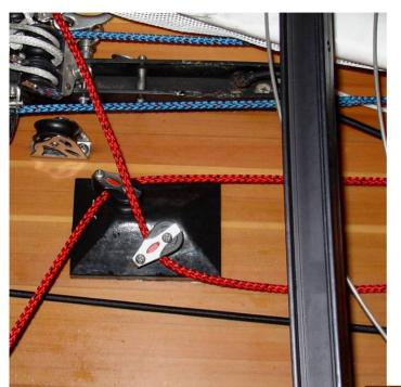
You'll need to make another bevel block like the two already installed on either side of the daggerboard case. You can see that it is located just forward of the jib turning block and about 2" away from the mast step on the starboard side. Install the two cheek blocks as shown. The line runs forward and attaches to a bullet block with the becket attached to the end of the forestay controll line
