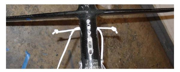
Pull the other line through from the other side and repeat the knot process. Remember, You can not get both lines through unless you leave them at the thin part until you are ready to pull both "home" at the same time.
