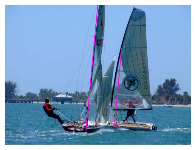
There is a situation when trapping high and carrying a lot of vang (like Unfortunate Events) that **the pressure on both primary shrouds goes nearly to zero.** The mast is being held up by the lowers, the trap wire, the windward cap the forestay and the wind. The high angle places enough pressure on the windward rail to offset the tripping moment of the daggerboard.
