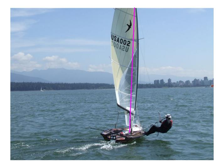
Here you can see that the spreader tip is forward of a straight line. That means that any further pressure in the upper mast pulls the mast tip aft and to weather. Again pulling on more forestay and letting off the primaries an equal amount (same total tension) would have straightened the lower mast and pulled the mast tip to weather—providing more power. If the waves had been any larger, that would have been important. In flat water it is a trade off between power and pointing ability.
