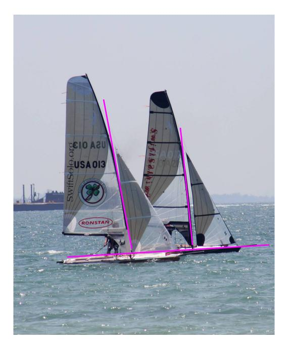
The lower masts are straight in both of these boats. Unfortunate events is reaching with the boom well out.
